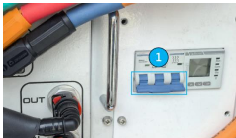
Figure 5-8: Turn off liquid cooling power switch
