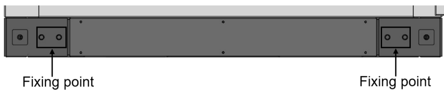
Figure 4-22: Fixing points of cabinet
