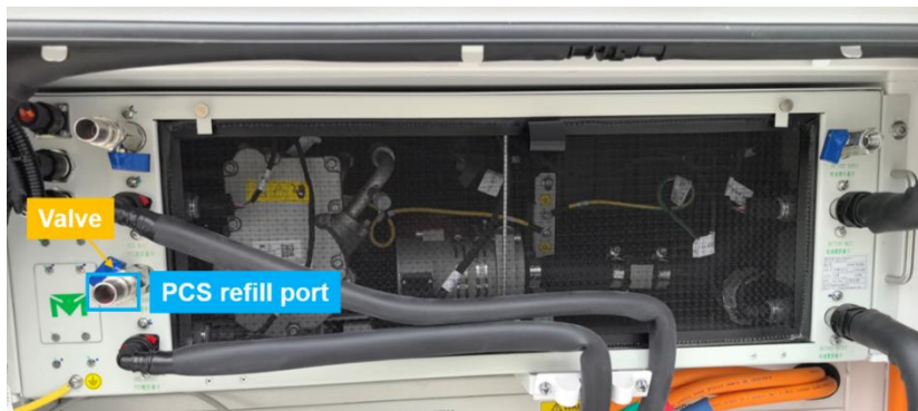
Figure 6-1: PCS refill port position
