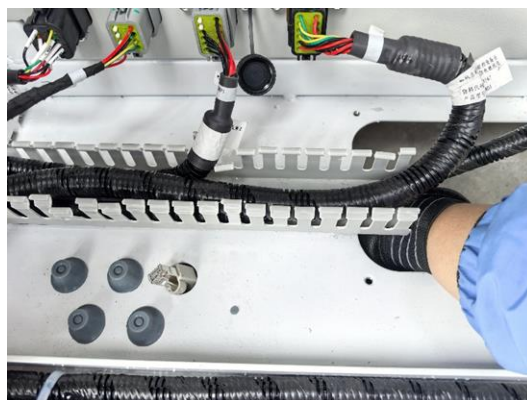
Figure 4-34: Routing communication cable
