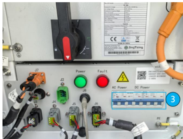
Figure 5-4: Turn on AC/DC switches
