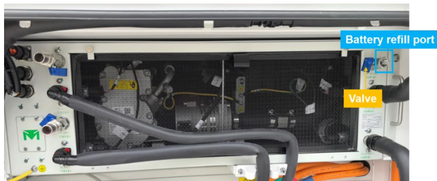
Figure 6-3: Refill port position of battery side
